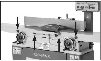
Figure 52. Front eccentric bushings.
